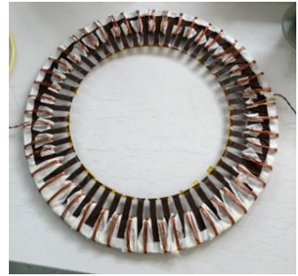
Fig1. Welded stator lamination stack
