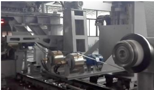
Figure1. Mass production of the material by a single-roller melt-spinning in B Plus Co.,Ltd.
