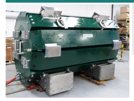
The magnet produces a homogeneous field profile over a large volume (Ø70cm x 200cm) The field is generated using four separately energisable circuits. Subtle changes in the field profile are possible by varying the currents in the four circuits.
