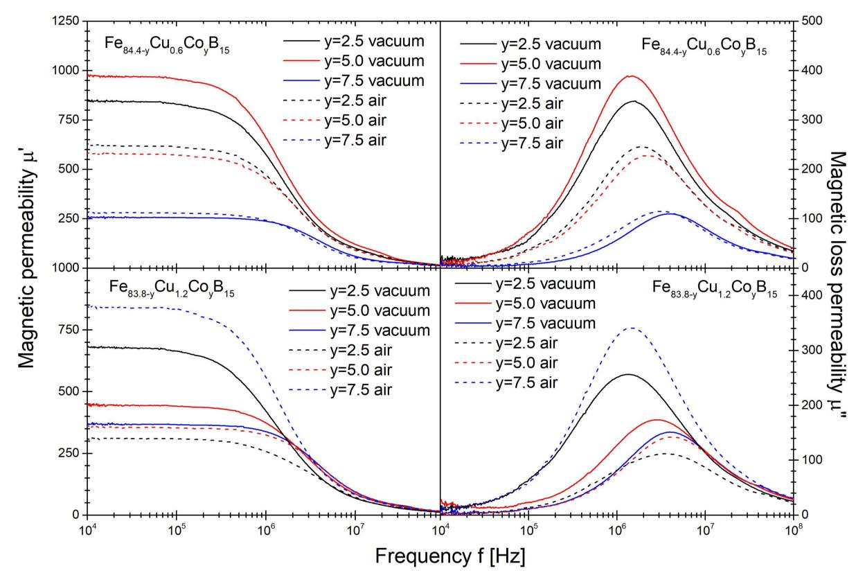
Magnetic permeability for samples annealed at the optimal annealing temperature in vaccum and air
