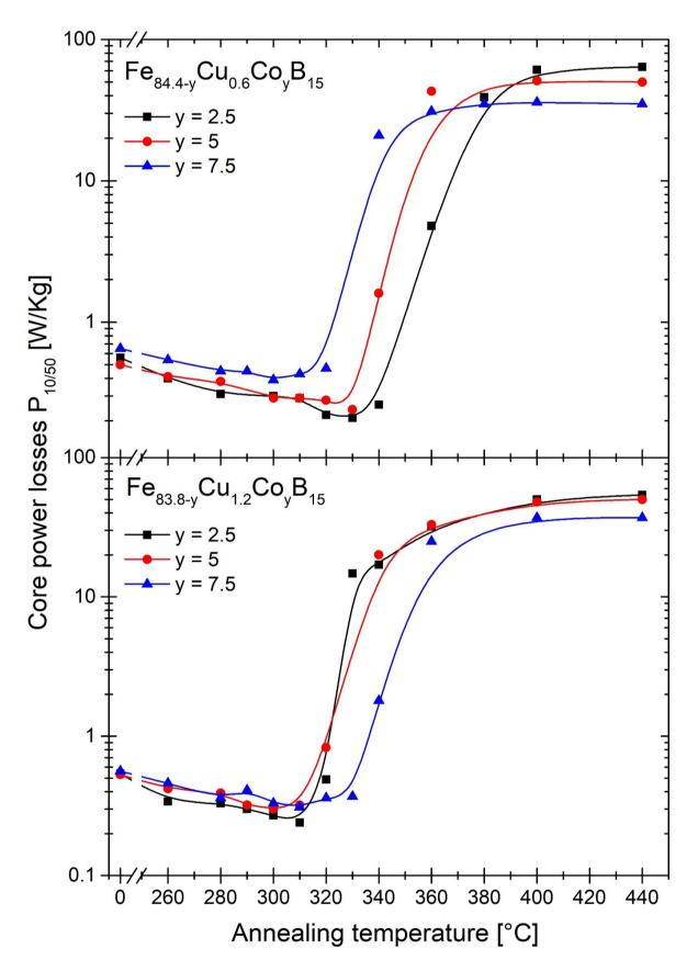
Magnetic properties: saturation induction Bs , coercivity Hc and core power losses Ps in a function of annealing temperature
