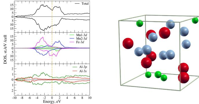
**Fig. 1.** Total and partial densities of states of the Heusler alloy  $Mn_{1.5}Fe_{1.5}Al$  (a). Optimized crystal structure with Al shown as small green spheres, Fe as big red spheres, Mn shown as grey spheres (b).
